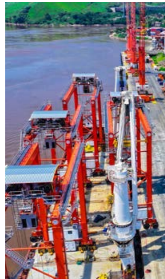
Matadi Gateway Terminal expanded its equipment fleet with two four new hybrid RTG cranes.
