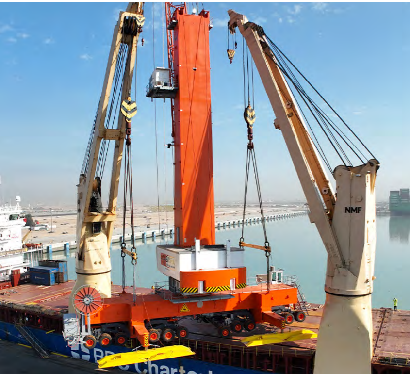
Basra Gateway Terminal's new mobile harbor crane
