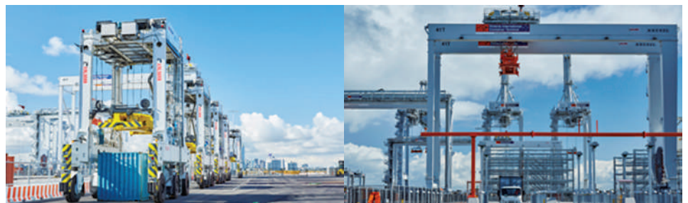
Kalmar Automatic Container Carriers (left photo) and Automatic Stacking Cranes in action at VICT
