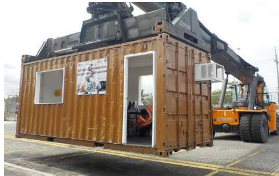
A reachstacker lifts a container converted into a make-shift office to simulate the actual shaking during an earthquake.
